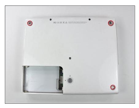
Remove the three newly-revealed Phillips screws.
