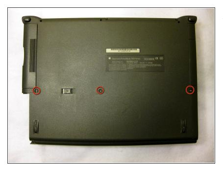
With the laptop upside down and with the battery removed, use a Torx #9 screw driver to remove the three .84 in. screws shown.
