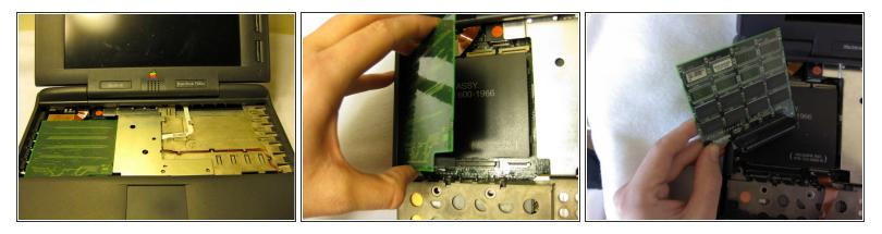
• Remove the RAM board located underneath the keyboard by carefully popping it out from its connection. Reinstall or replace as necessary.
