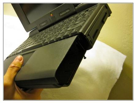
• The battery compartment is located in the front-right side of the laptop.
