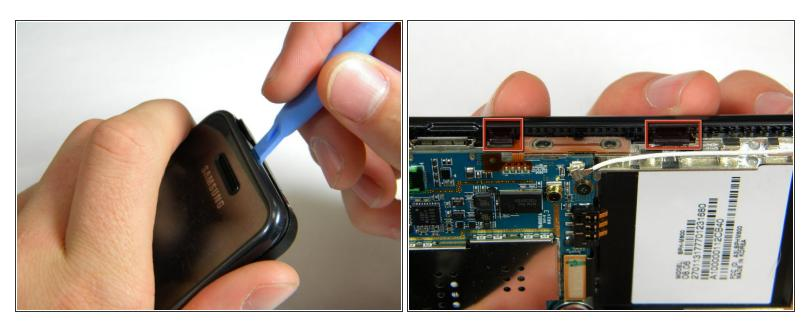
Use the plastic opening tool to unhinge the locks around the edges of the phone.
