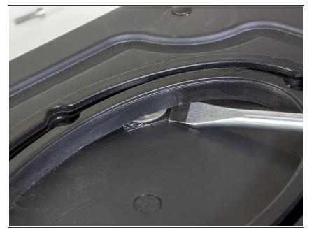
• Lift the oval rail slightly with the flathead screwdriver and replace the defective thread plate with the new one. Take care that the new oval thread plate is correctly inserted into the the rail.
