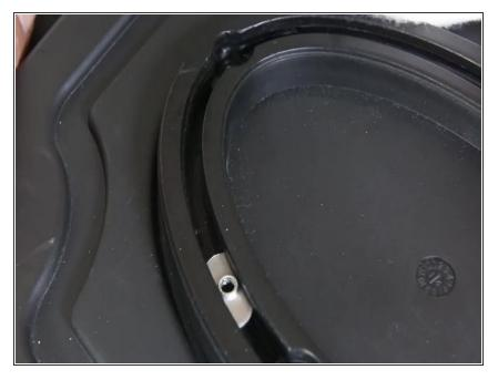
If the defective thread plate is still on the rail, it can be removed with the help of a 3 mm hex key. Use the hex key to push the thread plate into the marked section and push down.
