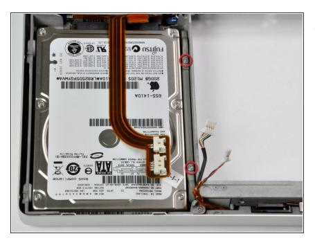
Remove the two silver Torx screws securing the hard drive bracket to the lower case.
