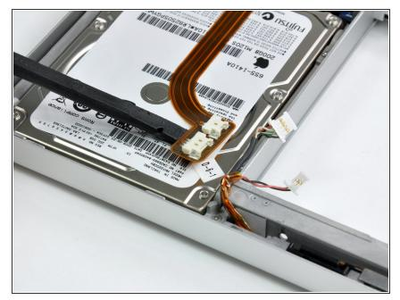
Using a spudger, carefully loosen the adhesive holding the ribbon cable to the surface of the hard drive.
