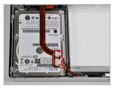
Disconnect the sleep light and IR sensor connectors from the ribbon cable on top of the hard drive.
