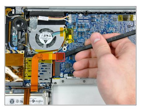
Disconnect the hard drive ribbon cable connector from the logic board.
