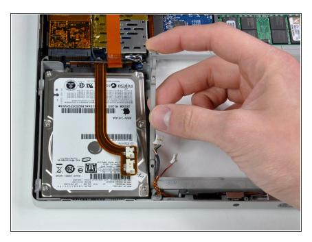
Remove the hard drive bracket from the lower case.
