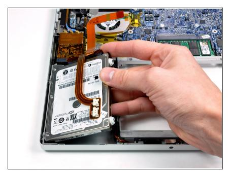
Lift the hard drive from the right side and pull it up and out of the lower case.
