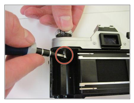
Open the film compartment and place the screwdriver in the the slot to keep the shaft from moving.
