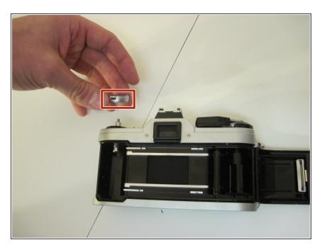
Remove the crank by rotating it counter-clockwise.
