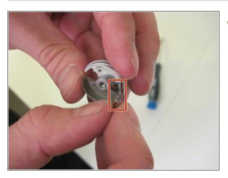
Remove the film rewind crank.
