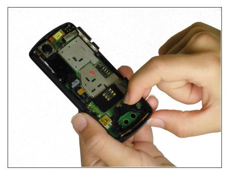
Lift the black rubber loudspeaker housing up and out of the plastic casing.
