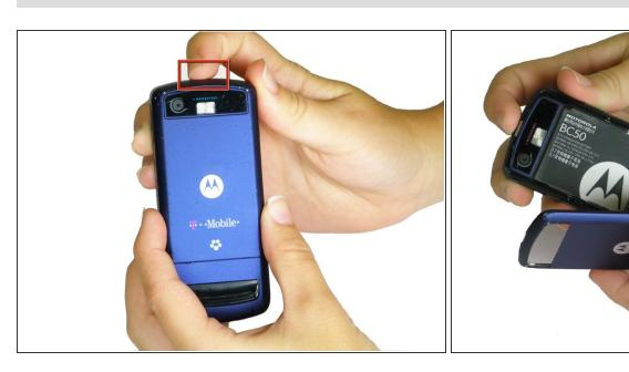
Press the panel release button on the top of the phone and simultaneously pull the rear panel away from the phone.
