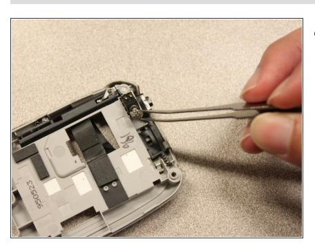
Use the tweezers to remove the vibrator module.
