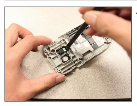
Use the spudger to pry out the camera flash module.
