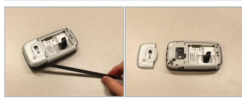
Work the <u>spudger</u> around the edges of the camera cover until it comes off.
