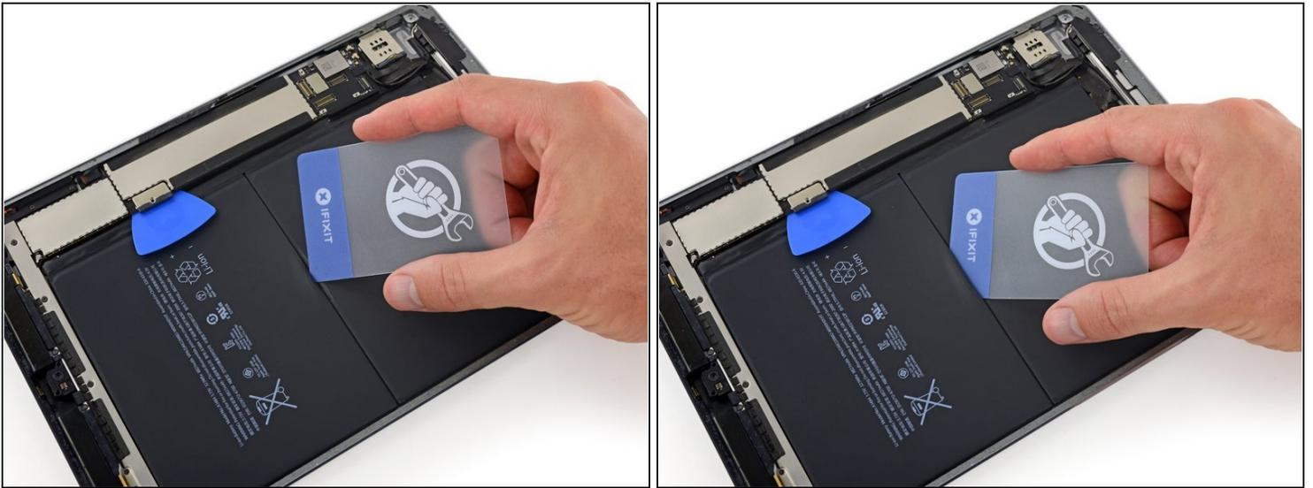
ⓘ In the following steps, you'll use [plastic cards](#) to separate the battery, which is glued to the rear case.
