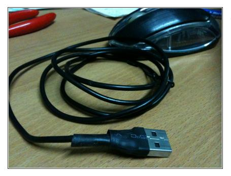
If mouse is working, use heatshrinkable tubing for close component and done.
