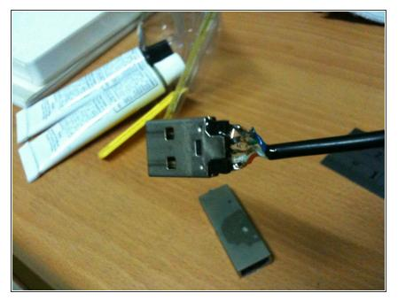
Soldering components together. In this case Red=Vol, White=Data -, Green=Data +, Blue=Ground.
