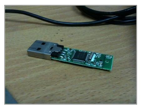
• Use soldering iron for take USB from flash drive.
