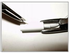
Carefully slice down the headphone jack connector with a sharp knife, being careful to not cut yourself.
