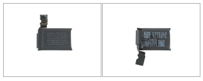
• With the glue stripped from the back of the battery, we get a closer look at its impressive specs. This cell is rated at 3.77 V and 273 mAh to yield a whopping 1.03 Whr of power.
