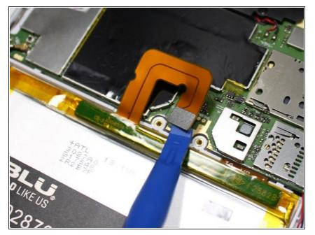
Disconnect the battery connector using a plastic opening tool or the flat end of a spudger.
