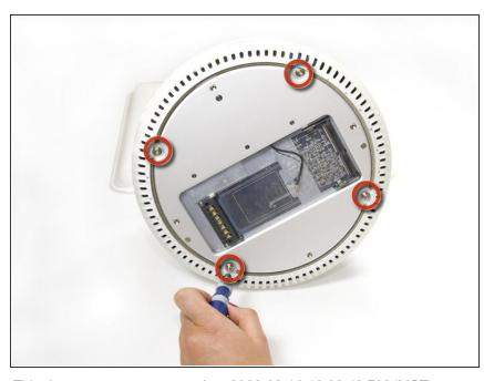
Remove the four 28.07mm Torx #15 screws from the lower case.
