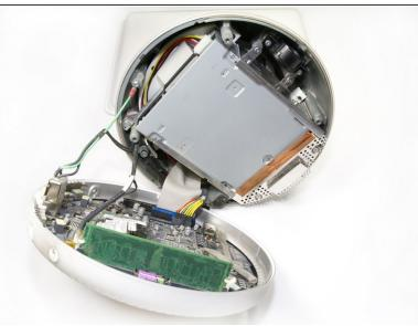
Open the base by carefully pulling straight off, do not rotate the cover.
