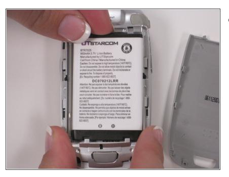
Carefully remove the battery from the phone by prying the battery from the top.
