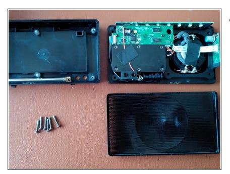
• Now the electronics can be removed from the carcass.
