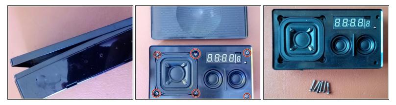
• Remove the six screws with a PH2 screwdriver
