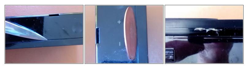
• The metal grille, in the front of the device by pry remove. Here is a thin plastic or metal object to use (in the picture is a letter opener to see), a coin is actually too thick. This can be a little hard!
