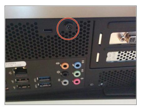
The first step is to unscrew this screw. After that you want to slide the case cover off of the computer.
