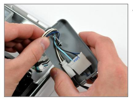
• De-route the inverter cables from the inverter cable cover hook.
