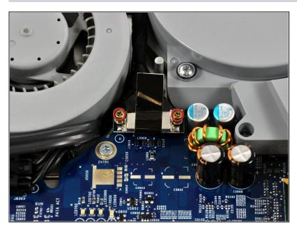
Remove the two 7.3 mm shouldered Phillips screws securing the display cable connector to the logic board.
