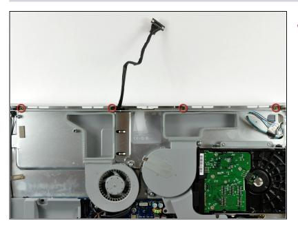
Remove the four coarse-thread
