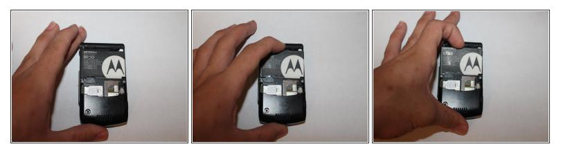
• Remove the battery by pushing down on it from the top while gently pulling it outwards.
