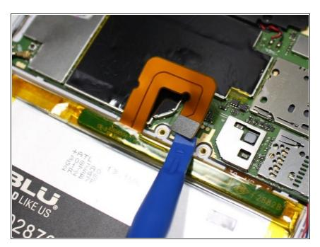
Disconnect the battery connector using a plastic opening tool or the flat end of a spudger.
