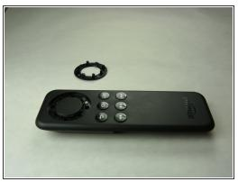
To remove the buttons use the blue plastic opening tool to pry out the outer ring.
