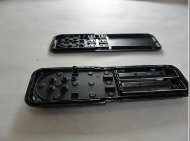
Remove top plate using plastic opening tools.
