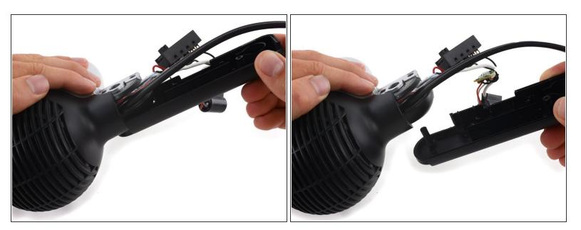
Remove the lower portion of the handle by sliding the peg out of the slot at the top of the handle.
