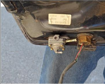
Carefully lift the tank up and off the frame of the bike, being sure that the fuel level sensor wire does not get caught in the frame.
