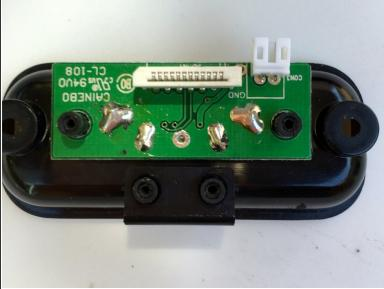
Remove the four 7mm Phillips #00 screws attaching the black plastic cover to the bottom of the adapter assembly.
