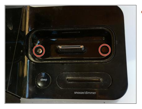
Remove the two 8mm Phillips #0 screws from the iHome's iPod adapter.
