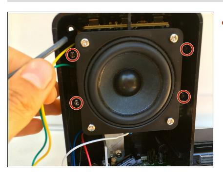
Remove the four 10mm Phillips #1 screws located on either side of the speaker.
