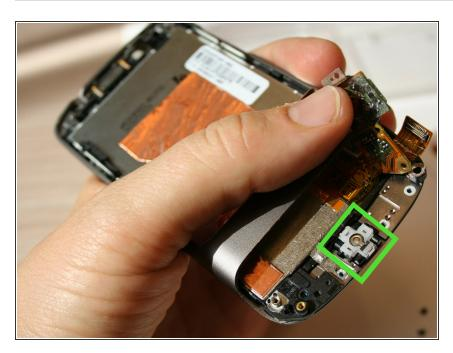
put the Trackball back in it's place: the 4 sides are not the same, one is different. Let this side point outwards
