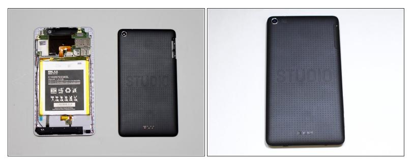
Once the back has been removed, you can snap the new one into place by pressing firmly around the edges with your fingers.
