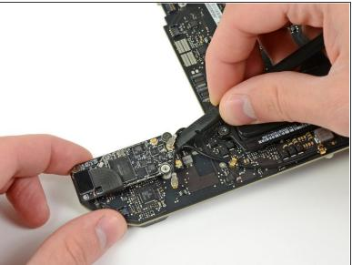
Use the flat end of a spudger to pry both antenna connectors up from their sockets on the AirPort/Bluetooth board.
