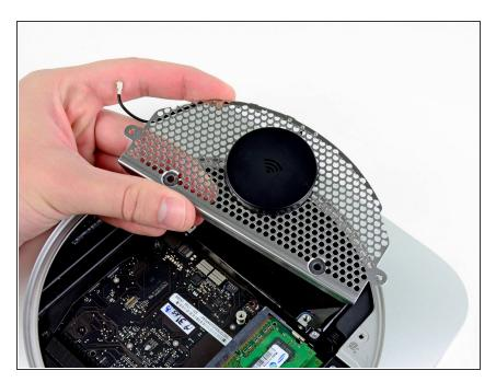
Remove the antenna plate from the mini.
