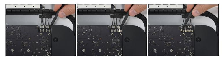
• Use a spudger to disconnect all four antenna connectors by prying them up from their sockets on the AirPort/Bluetooth Card
