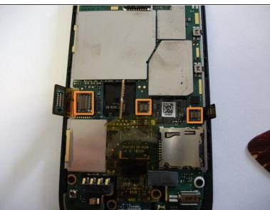
Use a spudger or a pry pick to release the 3 connectors marked in red in the photo. (The middle connector will be covered with a piece of tape.)
