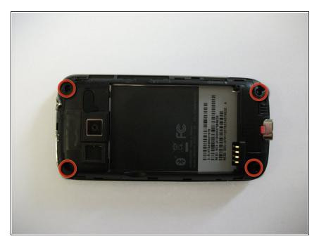
Use a T4 screwdriver to remove the T4 screws at the locations shown in red circles.
