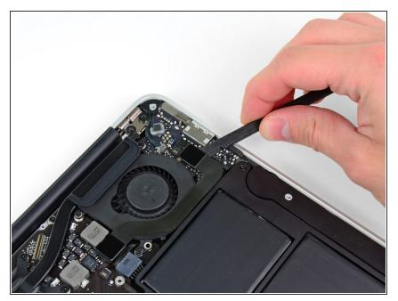
• Use the flat end of a spudger to pry the I/O board cable up from its socket on the I/O board.
