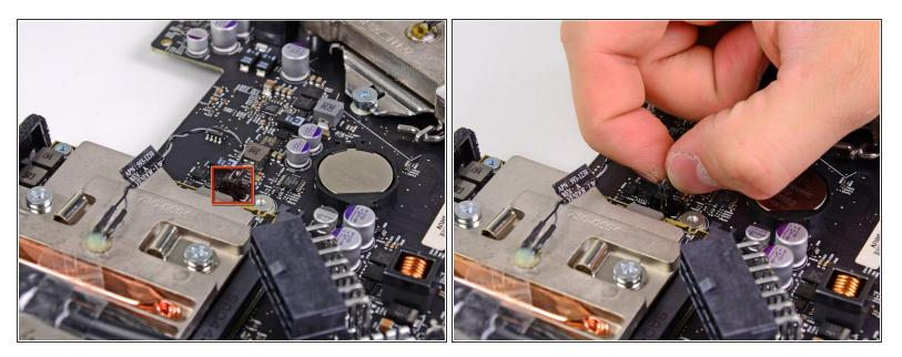
Grab the GPU thermal sensor cable connector and pull it straight up and out of its socket on the logic board.
