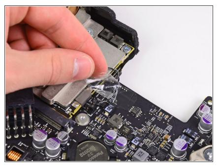
Remove the strip of tape securing the GPU thermal sensor cable to the logic board.
