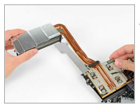
• Lift the GPU heat sink slightly and pull the GPU board out of its socket on the logic board.
