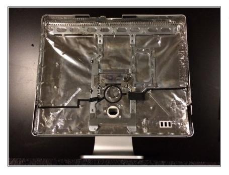
Firstly, I completely gutted the iMac, safely keeping the LCD screen to one side. I also repaired any torn EMI shielding and shielded all holes, with the exception of the power in, vent above this. (I also left the 3x USB ports free to fit a USB hub, but this didn't work great, so ended up being removed).
