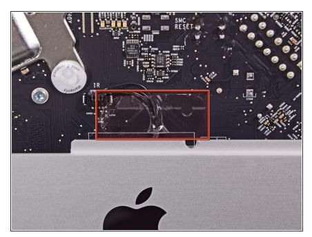
Remove the piece of tape covering the IR board cable.
