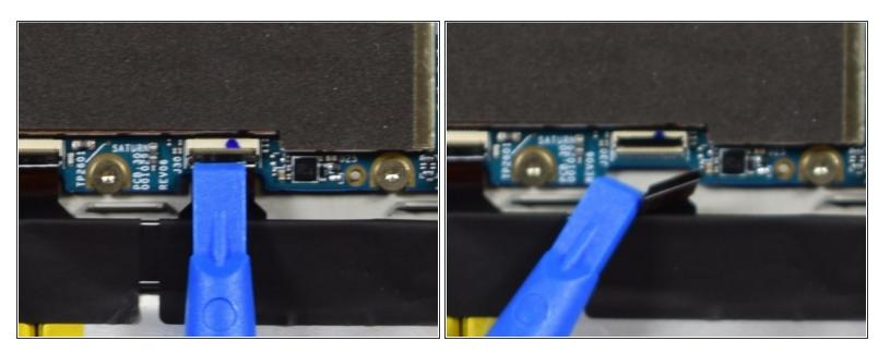
• Use a plastic opening tool to disconnect the ZIF connector by flipping up the black retaining flap.
