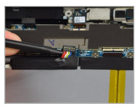
Use the spudger to lift up and release the battery connector.
