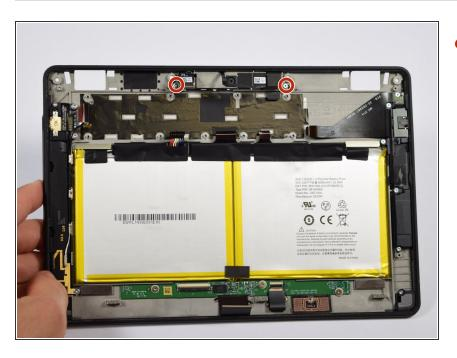
Remove the two 2.5 mm T5 screws.
