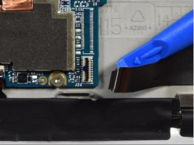
• Use a plastic opening tool to disconnect the ZIF connector by flipping up the black retaining flap.
