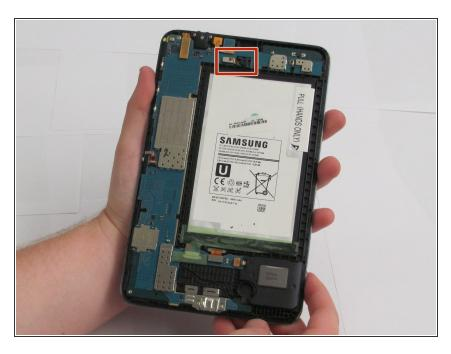
The rear facing camera will be located just to the right and below the front facing camera, near the top and center of the motherboard.
