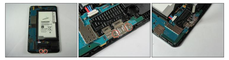
• Remove both 2 mm #000 Phillips screws from the metal charger port cover.
