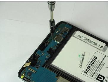
• Remove all three 2 mm #000 Phillips screws that fasten the mother board to the front panel.
