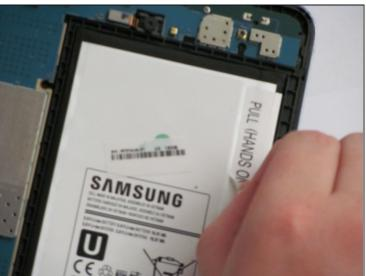
• Peel the sticker, reading "PULL (HANDS ONLY)," off of the battery starting at the detachable corner.
