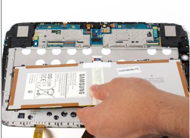
Disconnect the battery by lifting it upward and pulling it away from the connector.
