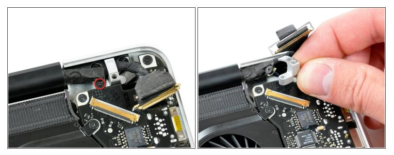
• Remove the 7 mm Phillips screw from the LVDS cable bracket.
