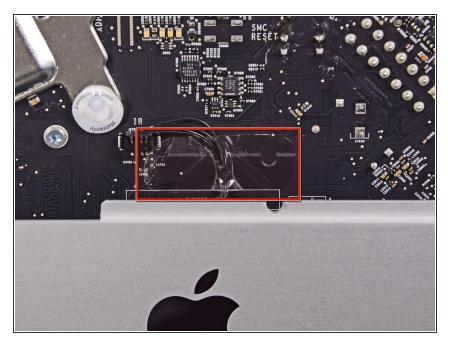
• Remove the piece of tape covering the IR sensor cable.
