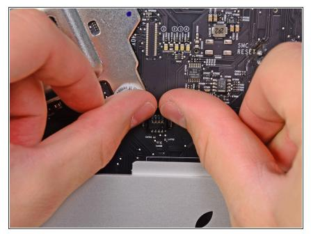
Use your thumbs to push the IR sensor connector out of its socket and toward the top edge of the iMac.
