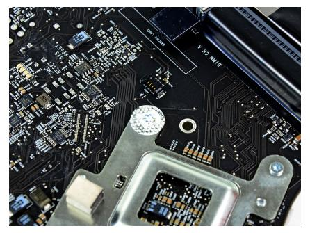
• If present, remove the "Warranty void if removed" sticker covering one hidden screw on the heat sink.
