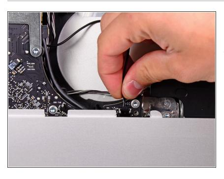
Pull the microphone cable connector toward the top edge of the iMac to disconnect it from the logic board.
