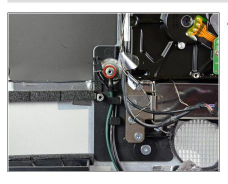
Use a 5 mm nut driver to remove the 15.7 mm long standoff securing the AC inlet ground loop to the outer case.
