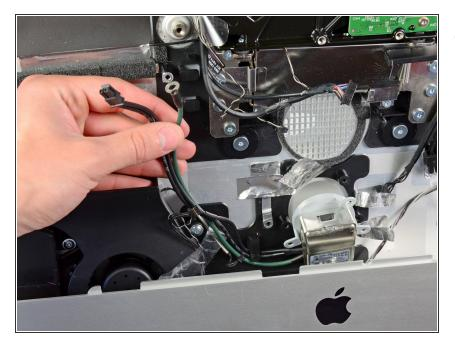
De-route the AC inlet and ground cables from their retainers in the outer case and remove the AC inlet assembly from the iMac.
