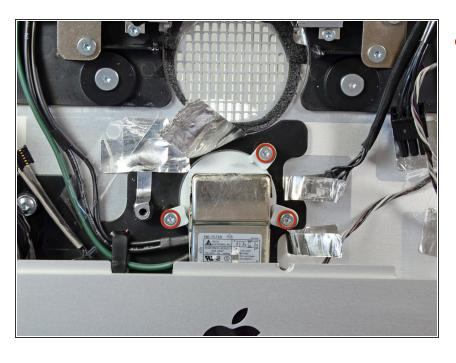
Remove the three 9.3 mm T10 Torx screws securing the AC inlet to the outer case.
