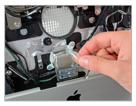
Remove the piece of clear tape covering the body of the AC inlet.
