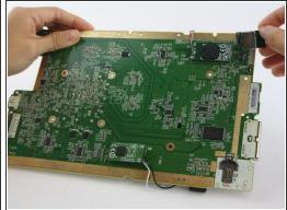
Pull up gently on the wireless modules to avoid breakage.
