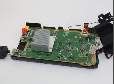
• Using a Phillips #1 unscrew all floor screws connecting the outer plate from the circuit board to remove the circuit board.
