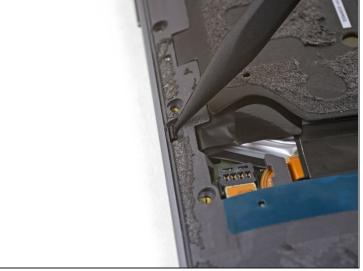
• Use the point of a spudger to push the small clip securing the left side of the midframe toward the edge of the phone, releasing the clip.
