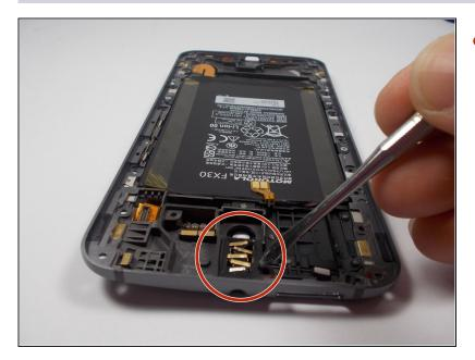
Using the nylon spudger, remove the auxiliary port.
