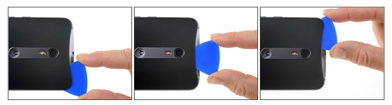
• Slice through the adhesive along the top edge of the phone, pulling the pick out slightly to guide it around the rear-facing camera.
