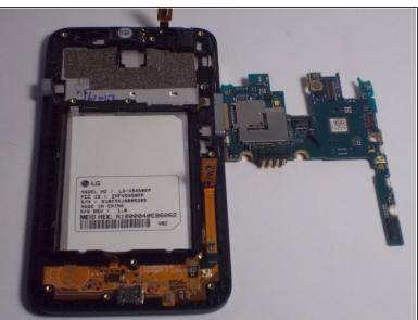
Push the blue lifting tool up underneath the logic board and pull it upwards removing it from the device.
