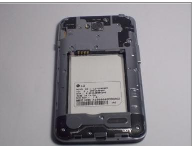
Flip the device over and remove the back covering.
