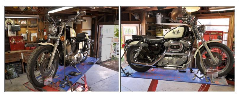
For the best access to the transmission drain plug, optimal draining, and accurate re-filling, we recommend working with the bike secured in an upright position.
