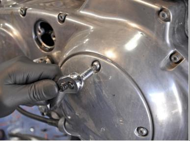
Using a T27 screwdriver bit, remove the four screws holding the clutch inspection cover in place.
