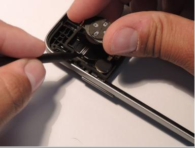
Use plastic tools to grab hold of one side of the speaker on the motherboard, and then gently lift.
