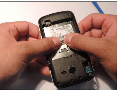
Unscrew the 1.2mm Phillip screw that connects the motherboard to the rest of the phone. Then by using your thumbs pop the inners of the phone out. Also use same J00 Phillips head bit from prior steps.
