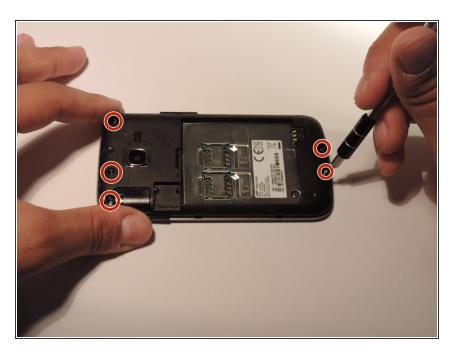
After following how to remove the battery, unscrew the five 1.2mm
