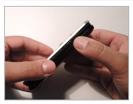
Place phone firmly between both hands with one hand flat on the back of the phone and pop off the back cover
