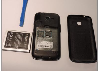
Once rear cover is off use small pastic spudger to lift battery out of the phone
