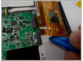
Remove the ribbon cable by lifting up on the connection with a plastic opening tool and pulling out the ribbon cable.
