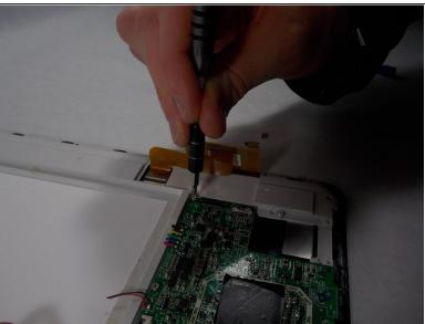
Use a Phillips head #0 screwdriver to unscrew the 5 philips head screws labeled in BLUE.
