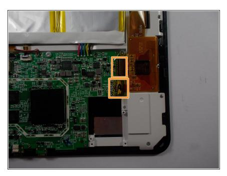
Peel off the tape covering the two connections labeled in orange.
