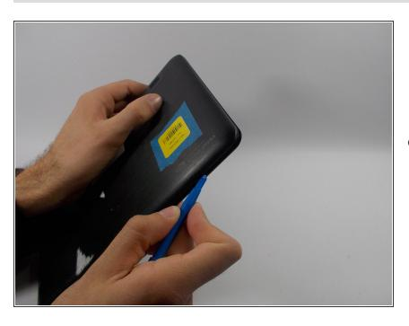
The rear panel is secured to the front case by 26 clips attached to the rear panel. These clips lock onto
